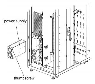
6 Slide the new power supply into the opening and tighten the thumbscrew.
