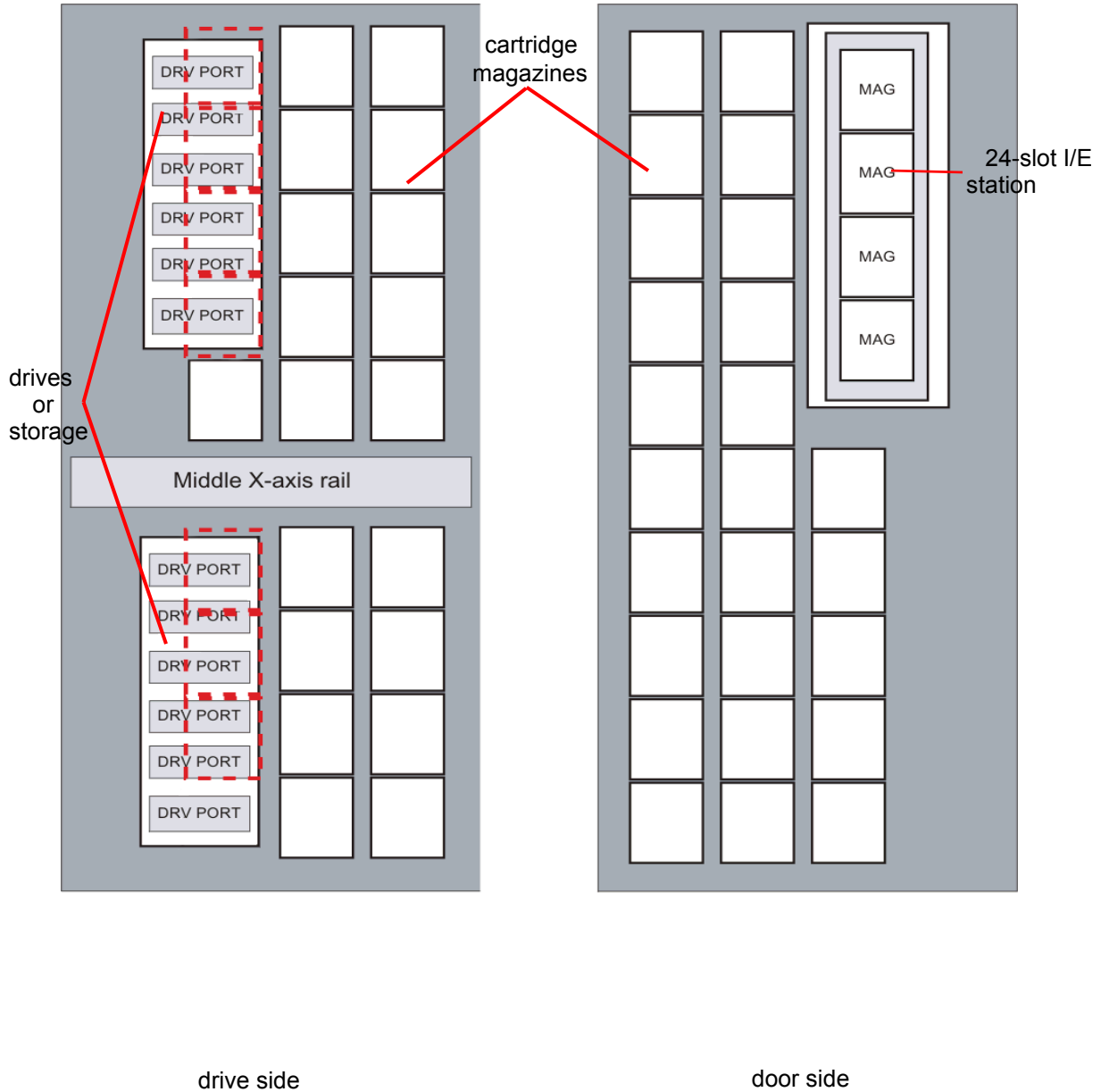
Figure 5 Magazine and Drive Location in the Single-Robotics Control Module
