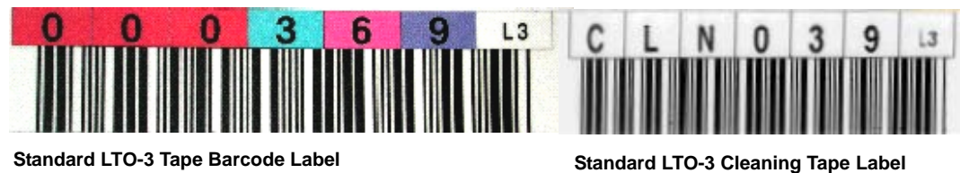
Figure 5 Standard LTO3 Tape Labels
