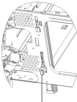
Y-rail in unlocked, functional position
