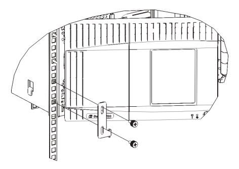
13 If the module you are installing is an expansion module, engage the Y-rails of the new module in your library configuration. Ensure that the Y-rails are properly aligned, and that the thumbscrews are tightened.
