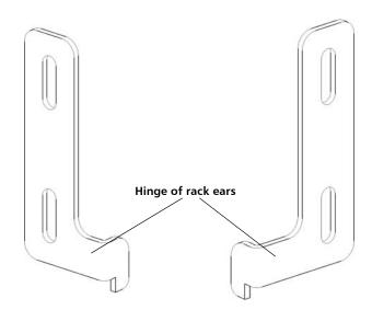
**b** Using two M5 thumbscrews, fasten the rack ear to the rack, as shown below. The thumbscrews should thread through the nut clips (or cage nuts) and fasten completely and evenly.
